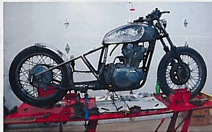
Steel lunch box mounted on the lower frame hides the bike's wiring and electrical components. (above)
